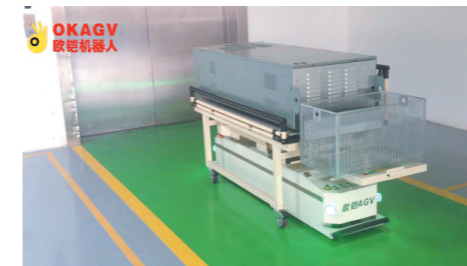
激光潜伏AGV待进入电梯 Laser guided AGV enter& exit elevator
